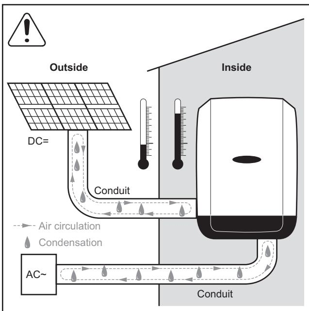
**NOTE!** Condensation within the conduits can damage the inverter or components of the photovoltaic systems.
