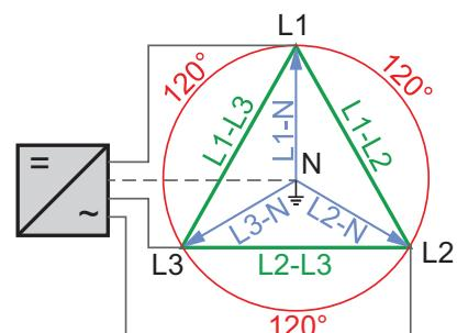
**Hi-Leg Delta** Neutral conductor necessary
