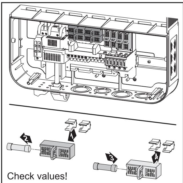
EN-US: To avoid the risk of a fire, only replace faulty fuses with new ones of the same rating.
