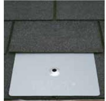
4. Use the EJOT Click&Drill hole-saw tool with end position stop to drill the pilot hole (15/64" diameter - 6.0 mm) in the roof and rafter for the lag bolt and the counter hole in the upper shingle (thickness up to 1/8").
